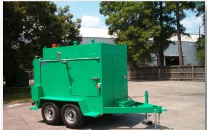
A compact fully enclosed hydrostatic test unit featuring its own tool box, water and fuel supply tanks
